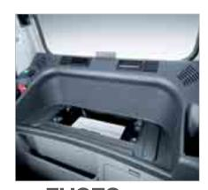
The fuses are inside the cab, protected from dust and water as well as easy to reach and control.
