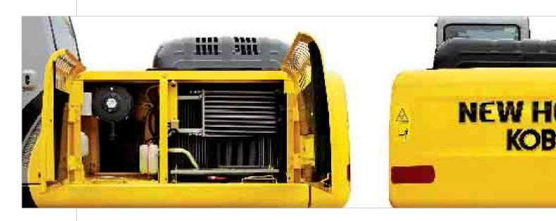
he simplified layout of all vital components of the New Holland E215B under both the right and the left side panels makes maintenance much easier, less time consuming and less costly, and provides much better access for servicing. There is plenty of room in all compartments and most components are positioned in such a way to enable easy access from ground level. **An elegant and modern design added to state-of-the-art technology.**
